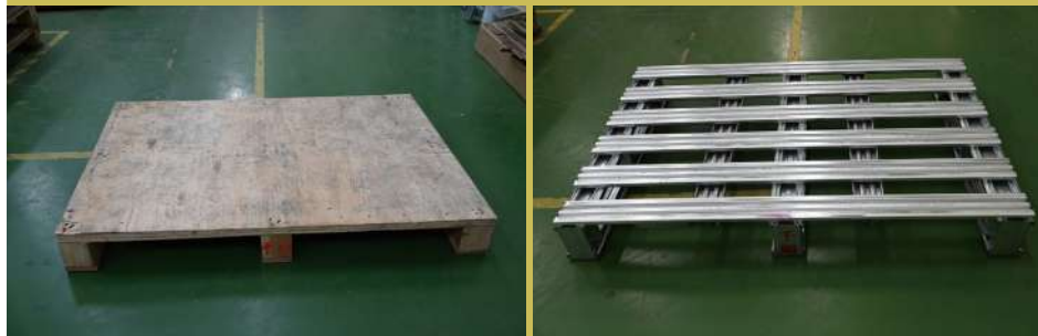
▲ The existing wood pallet material used in the Taiwan plant is changed to a light steel pallet, which is beneficial for reuse and re-circulation.
